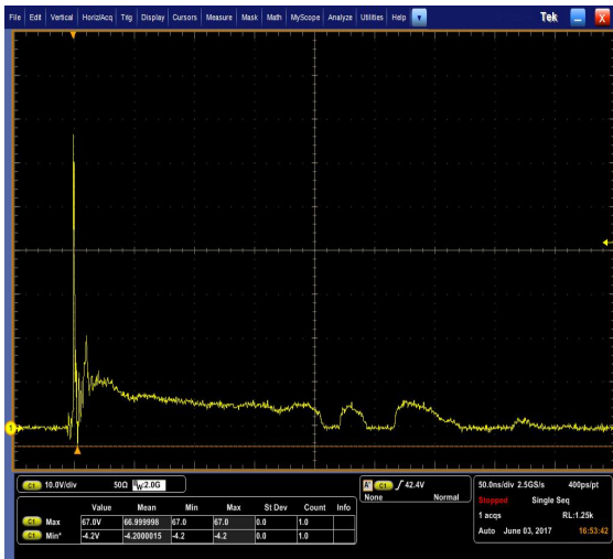
Fig1. ESD Clamping Voltage Screenshot Positive 8 kV Contact per IEC61000-4-2
