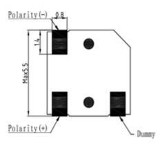
\*Unit: mm; Tolerance: ±0.3mm Except Specified
