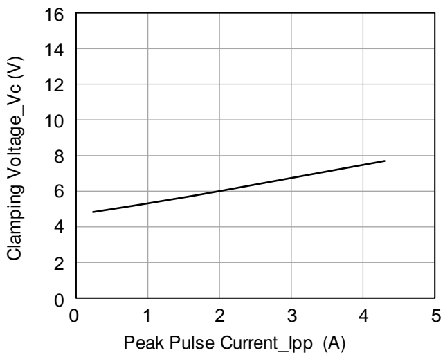
Figure 3. Clamping Voltage vs. Peak Pulse Current according to IEC 61000-4-5.
