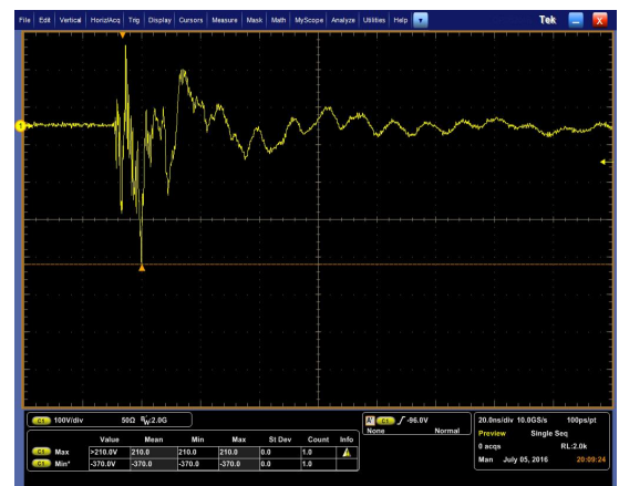
Figure 6. ESD Clamping Voltage Screenshot Negative 8 kV Contact per IEC61000-4-2
