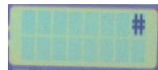
Figure 4 Display example of the LCD after touching capacitive switch key [TSW12] of the ML62Q1367 Capacitive Switch Application Board.
